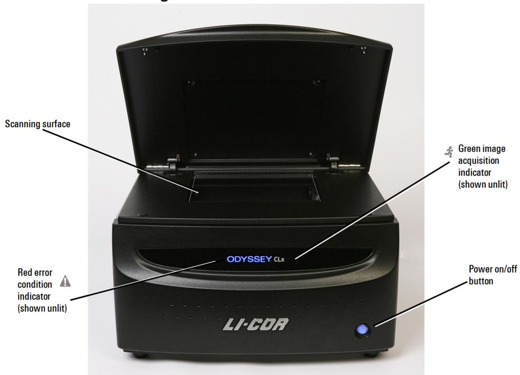
Figure 2-1. Front panel features and power button on the Odyssey CLx.
